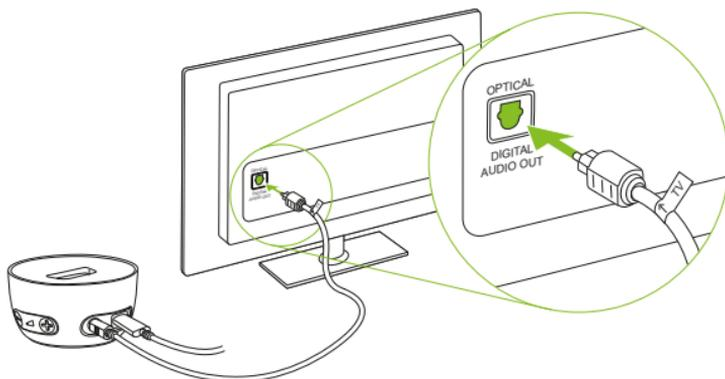
**i** Protect your eyes of the optical light from the optical Toslink cable when plugged into the device or TV.
